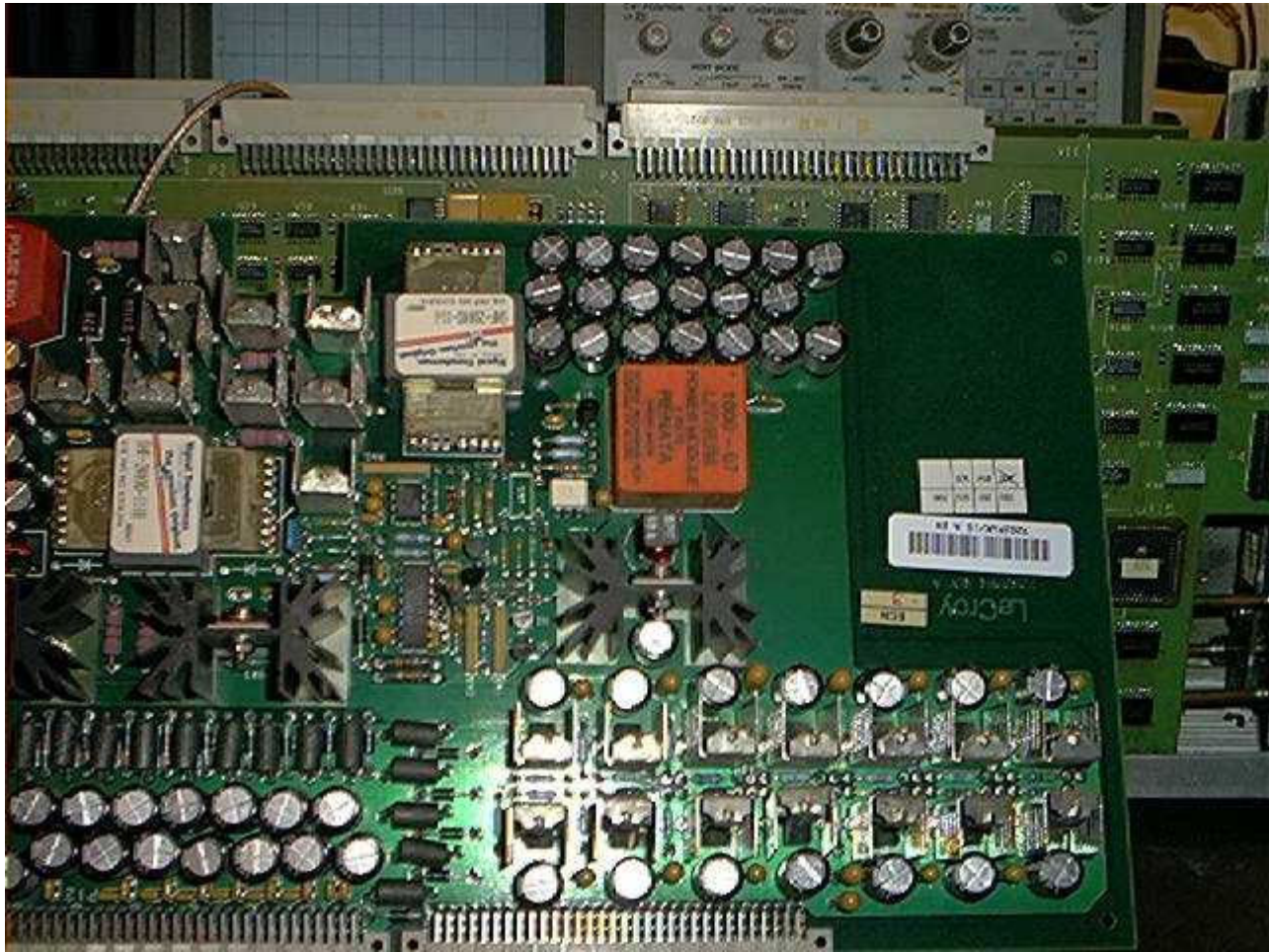
Showing the lithium battery (orange colored block).
